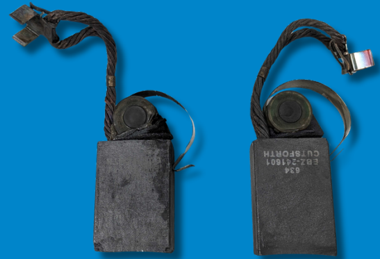
Melted sensors on the brushes
