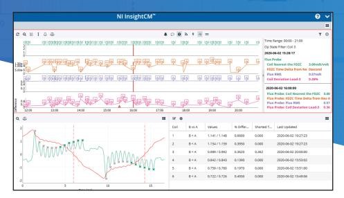
Rotor Flux monitoring (RFM) acquires signals from variances in the magnetic flux within a generator to indicate deterioration of winding insultation resulting in shorted turns. This damage can lead to:
