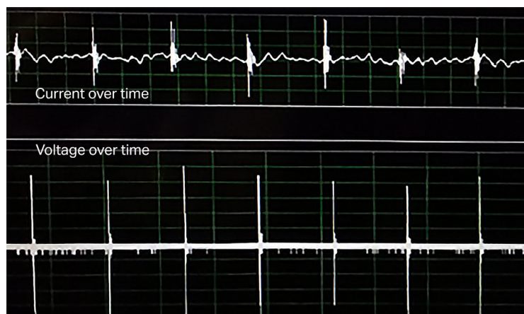
Figure 1) Example of an expected shaft grounding current and voltage waveforms over time.
