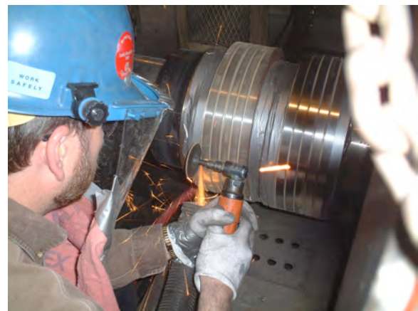
Figure 20: Ring Re-Grooving (Cutsforth Inc. Patented process)
