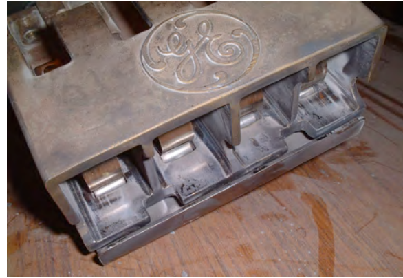
Figure 8: Carbon Deposits, Plated Holder
