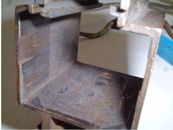
Figure 17: Brush Box Erosion
