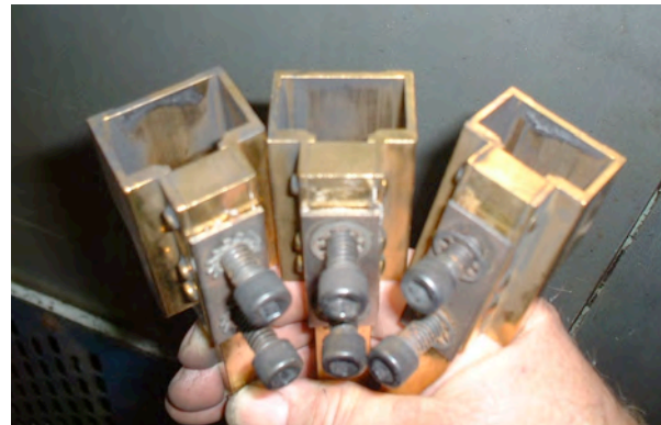
Figure 9: Carbon Deposits, Un-plated Holders
