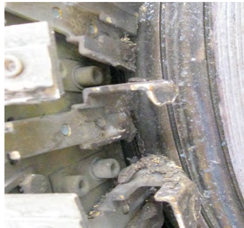
Figure 7: Molten Brush Holders
