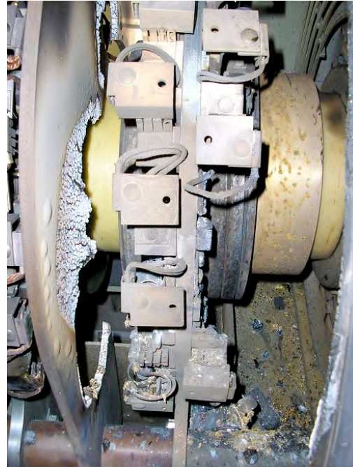
Figure 4: Effects of a Collector Ring Fire
