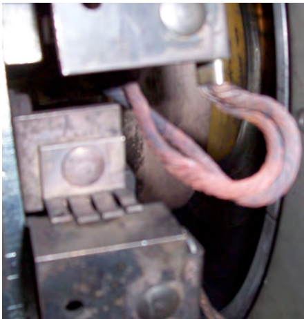
Figure 18: Indication of Selective Action due to Lead Discoloration
